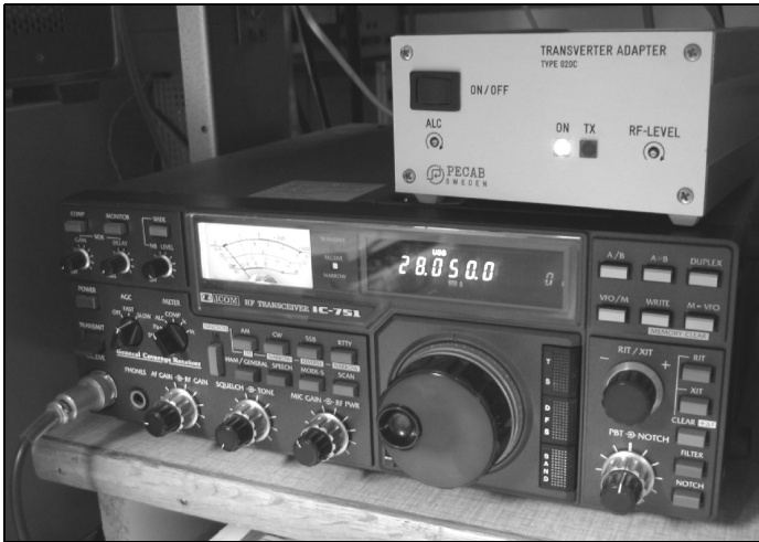
Fig 1: Picture of the transverter adapter in use with an ICOM IC751.
